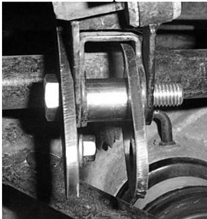
6. Connect the top of the shock to the lift brackets using a 10mm x 50mm bolt and one 10mm washer between the shock eyelet and the bracket.
