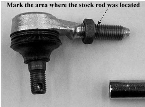
3. Once you have marked both tie rod ends remove the stock tie rod and ends from the ATV.
