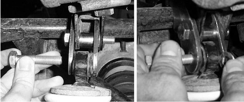
7. Secure brackets using at 10mm lock nut provided in the kit.
