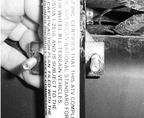
4. Connect the name plate to the backing plates using 1/4" washers and 1/4" lock nuts.
