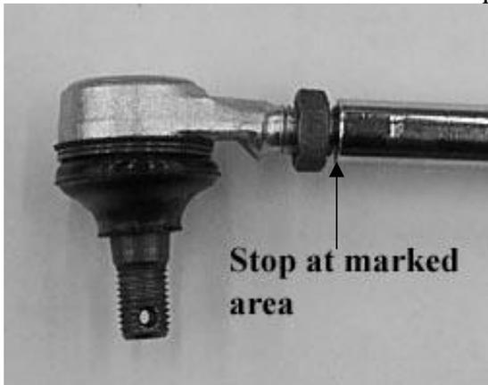
8. Install the new tie rod assembly onto the ATV.
