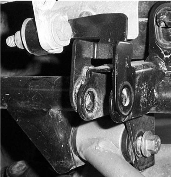
4. Place the rear long bracket on the outside of the shock mount to the side that is to the front of the ATV. Insert a Spacer into the shock mount tabs secure the brackets and spacer using a 10mm x 50mm bolt and 10mm lock nut.
