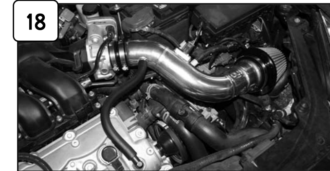
The installation of your Takeda performance intake is now complete. Please check all components and re-tighten if necessary. Thank you for choosing Takeda!
