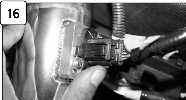
Re-connect MAF sensor harness.
