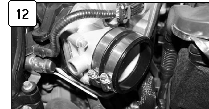
Attach coupling to throttle body using provided clamps. Do not tighten.
