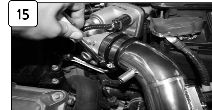
Tighten all clamps using 5/16" nut driver.
