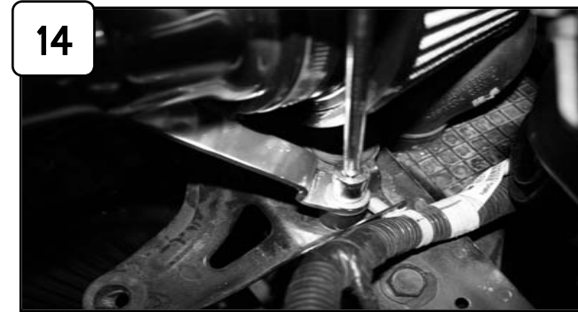
Using provided flat washer and nut, secure tab using 13mm socket or wrench.
