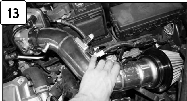
Install intake assembly and position tab to isolation mount. Do not tighten.
