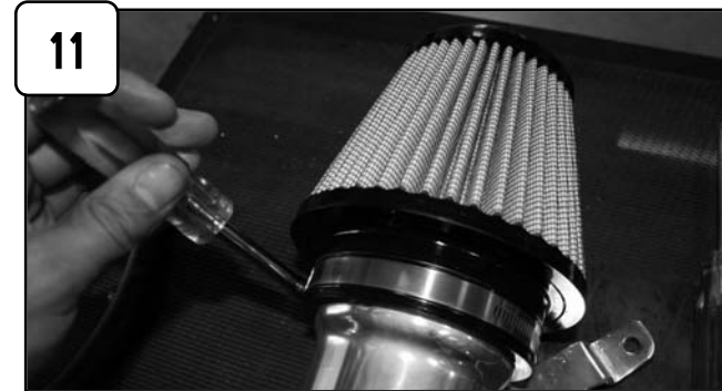
Attach air filter and tighten using 5/16" nut driver.
