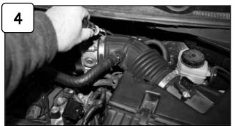
Disconnect MAF sensor harness. Loosen clamp on throttle body.
