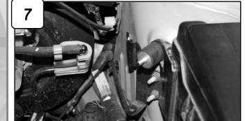
Install M6 male/female isolation mount to ECU harness bracket and secure.
