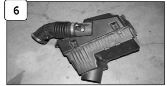
Remove stock intake out of vehicle.
