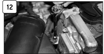
Loosen screw holding ECU wire harness. See step 13.
