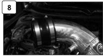
Attach coupler with clamps to tube. Do not tighten.
