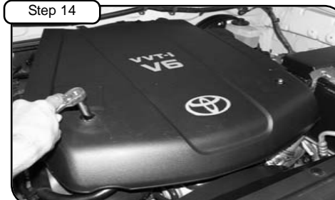
Temporarily install engine cover and position tube to align stud from step 12. Tighten coupler clamps and then tighten engine cover nut using 10mm socket.
