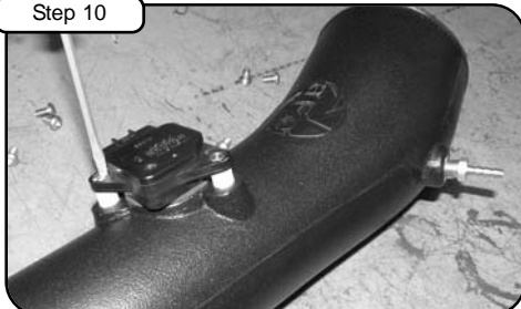
Remove MAF sensor from OE airbox using phillips screwdriver. Re-install to new aFe tube with hardware provided (make sure gasket and nylon spacers are between tube and sensor) using flat head screwdriver. Install brass hose fitting.
