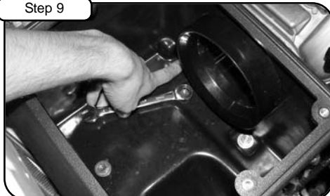
Place housing in to vehicle and tighten using 12mm socket or wrench. With M8 nut & washer provided tighten down housing on to isolation mount with 13mm wrench.
