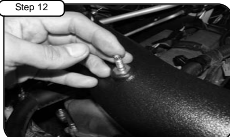
Remove M6 insert from OE air box, loosen using adjustable wrench. Re-install on to new tube and tighten. Connect large vent hose and connect small vent hose (5/32" hose provided) between tube and fuel regulator.
