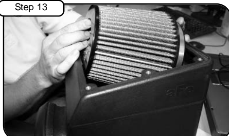
Place high FLOW filter into housing and tighten using 5/16" nut driver. Place cover on to housing using button head screws provided, tighten using 5/32" allen key. (place filter into housing at slight angle)
