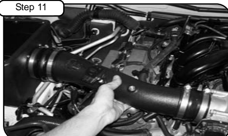
Place couplers on to tube with clamps provided, and install loose to allow repositioning.
