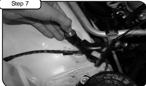
With 10mm socket with extension, remove bolt holding AC bracket. Insert M8 isolation mount and hand tighten firmly. (It may be necessary to clean the threads of undercoating or paint)
