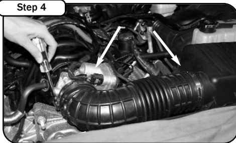
Step 4 Loosen the two hose clamps on the intake duct and remove duct form engine bay.
