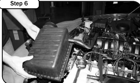
Step 6 Remove the 5/8" breather hose on the side of the valve cover. Remove airbox assembly out of the engine bay.
