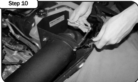
Step 10 Align the mounting holes on the tube and the housing. Secure the assembly with the provided M6 bolts washers and nuts.
