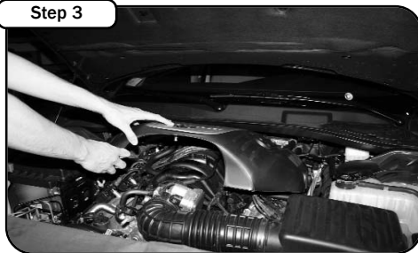
Step 3 Disconnect negative terminal from battery. Lift off Hemi engine cover. Remove the Temp.Sensor on the side of the intake duct. Be careful not to damage sensor
