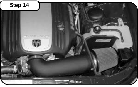
Step 14 Place enclosed CARB EO sticker on a clean/smooth surface on or near the intake system. EO identification label is required in passing the Smog Check inspection. Your installation is now complete. Tighten all connections and clamps. Re-check after a few hours.
