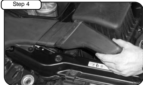
Step 4 Remove front snorkel from ducting to stock airbox.
