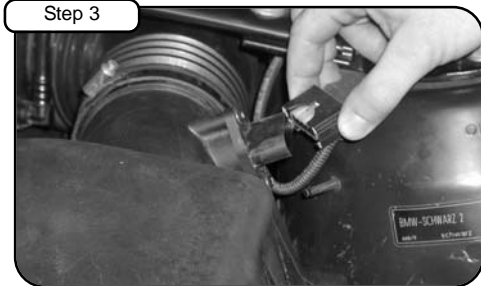
Step 3 Remove factory harness from Mass Air Flow sensor and place out of the way until re-assembly.
