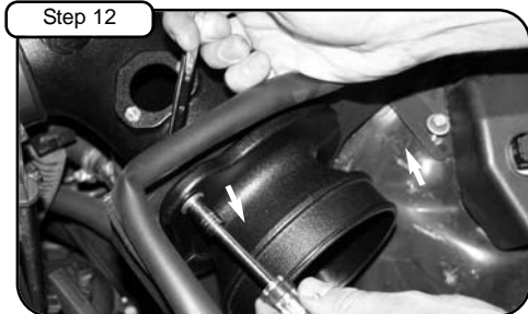
Step 12 Align two holes on tube flange to holes on housing. Use provided M6 hardware to mount tube flange to housing.
