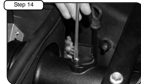
Step 14 Install Mass air flow sensor onto tube using provided gaskets, spacers and screws.
