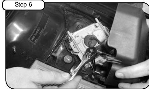
Step 6 Remove plastic cover from headlight controller via locking tabs. Using a 10mm socket, remove the (2) bolts securing controller to allow for its movement and to release lower half of airbox.
