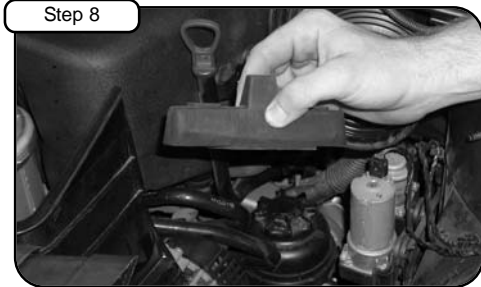
Step 8 Remove rubber mount from tab beneath factory airbox.
