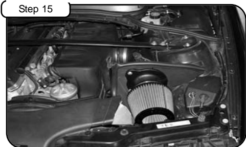
Step 15 Make sure all hoses and clamps are tight and that all electrical components (if applicable) are secure. Check and retighten connections and filter after a few hours of operation.
