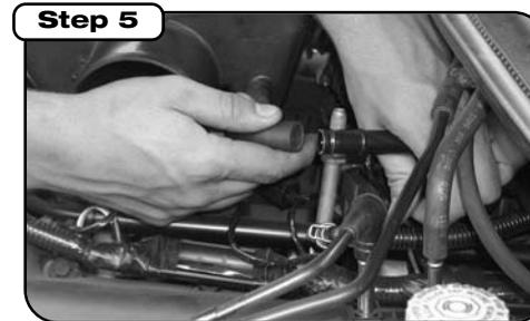
Remove vent hose at tubing coupler.
