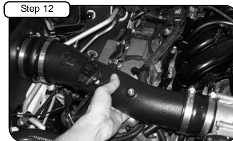
Place coupler 05-00794 with clamps #072 onto tube for adaptor side of housing. Then place coupler 05-00815 with clamps #052 and #048 onto tube for throttle body side. Install loose to allow repositioning.
