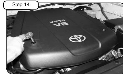
Temporarily install engine cover and position tube to align stud from step 13. Tighten coupler clamps and then tighten engine cover nut using 10mm socket.
