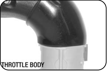
THROTTLE BODY Position coupler and clamps over throttle body (3.5" x 4.0") (clamps removed for clarification). The smaller (3.5") end of the coupler goes over the throttle body. The (4") end of the coupler goes around the intake tube.
