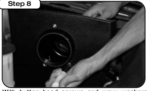
Step 8 With button head screws and wavy washers install filter injection molded adapter. Tighten using 5/32" allen key.
