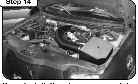
Step 14 Your installation is now complete. Check after a few hours of operation all hoses and clamps are tight and that all electrical components are secure. Thank you for choosing aFe!
