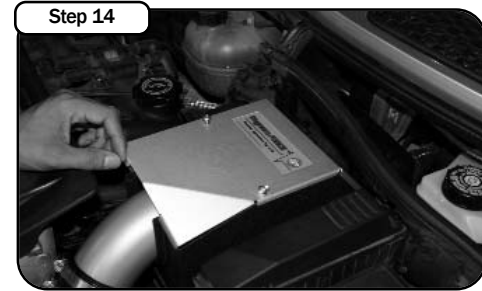
Step 14 Place the housing lid over the housing, secure with the supplied button head screws.
