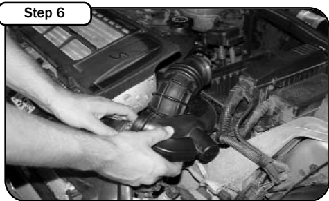
Step 6 Remove the OE intake duct, set to the side for later use.
