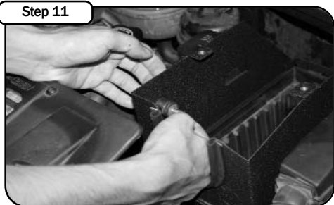
Step 11 Install the rubber isolation mount on the side of the housing. Use the supplied washers and nuts. Re-install the OE intake duct.
