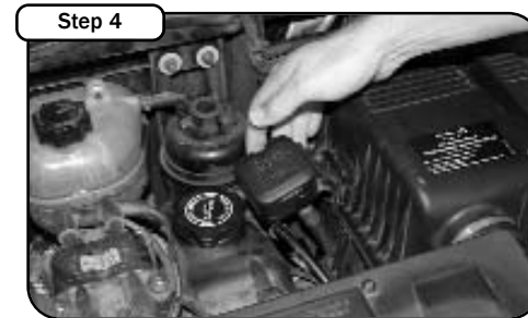
Step 4 Remove the positive terminal from the side of the air box. Lift up and out and carefully set to the side.
