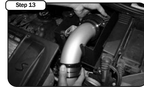
Step 13 First place the tube in the housing and secure to the isolation mount. Second slide the coupler over the intake tube. Tighten clamps and secure tube to housing with supplied nut and washer.
