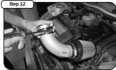
Step 12 Install the pre oiled air filter on the intake tube. Slide the coupler and clamps on the intake tube. Do not tighten clamps at this time.
