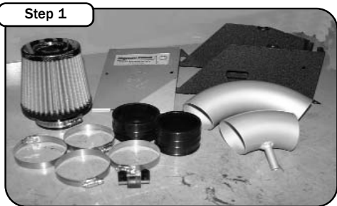
Step 1 Complete intake system. Please verify all parts are present prior to installation.
