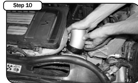
Step 10 Slide the smaller coupler and clamps over the throttle body. Insert the intake tube with the breather nipple in the coupler. Re connect the breather hose to the nipple.
