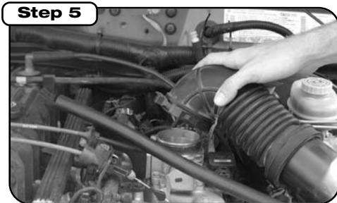
Loosen clamp at throttle body and remove.
