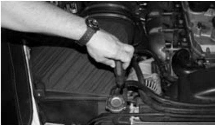
1 – Disconnect negative (-) battery terminals from BOTH batteries. Remove air intake turbo inlet from the vehicle.
