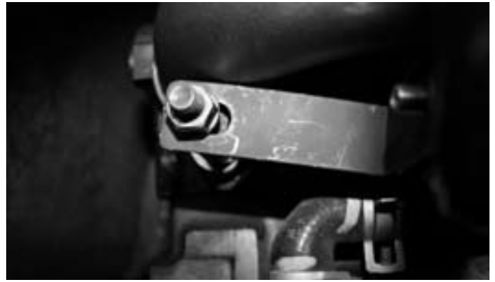
13 – If using bracket provided, install on bolt farthest to the back of the manifold after bolts are tightened.
