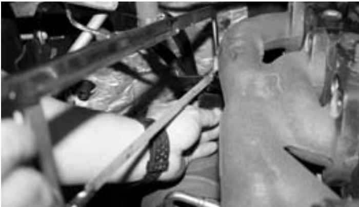
3 – Disconnect the water line bracket from the manifold. It can be very difficult to remove. An option is to cut the bracket and use the supplied bracket parts for later installation.
