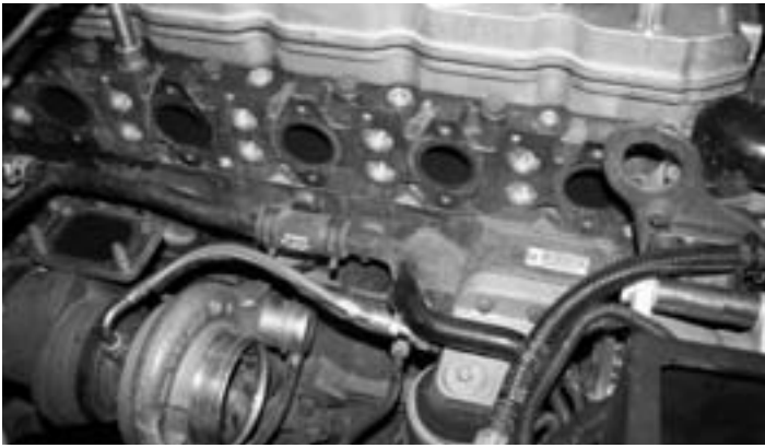
9 – If turbine housing has long shouldered studs (approx. 1" shoulder), remove them and replace with studs provided. NOTE: aFe will not replace turbine housings if damaged during stud removal.
