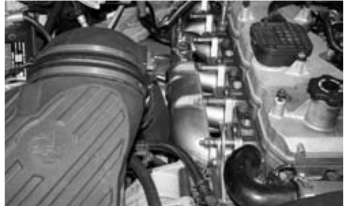
15 – Re-install heat shield and air intake turbo inlet. Reconnect the negative (-) battery terminals. Your installation is complete. Thank you for choosing aFePower!
