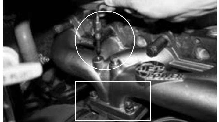
14 – Use anti-seize on turbo mounting studs and torque nuts to 32 ft-lbs. Re-install the EGT sensor. Install 1/8" NPT plug supplied into open port.
