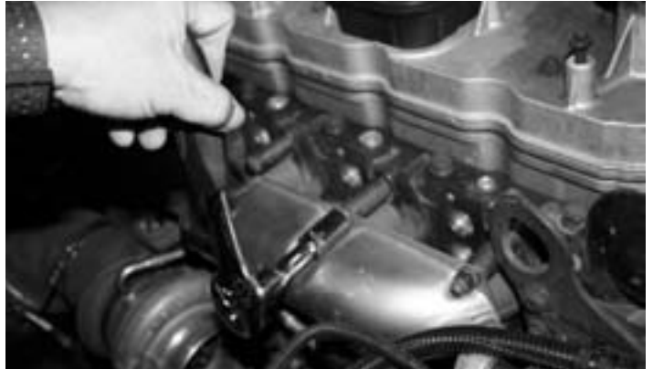
6 – Remove 4 nuts holding the heat shield.
