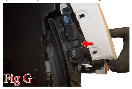
10. Using a 10mm Socket, remove the air dam mounting bolts (x3). Then, remove this air dam from the vehicle
