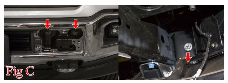
4. Remove the OEM Bumper from the vehicle.
