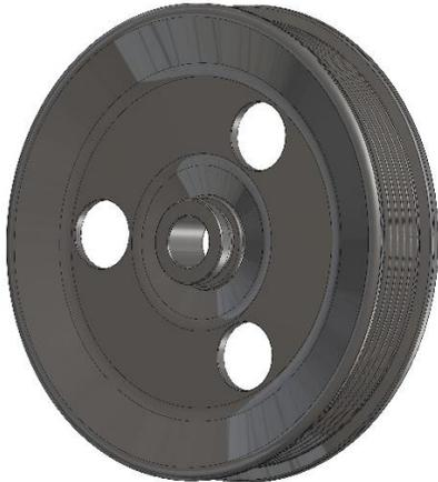
**Power steering pump pulley**
