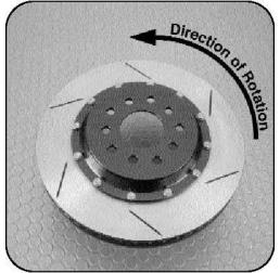
Non-modified or plain rotors that employ a curved vane design <u>must also</u> rotate in a specific direction. The curved vane rotor is designed to draw air into the center of the rotor and force the air to exit from the outer edge (see diagram on left).
