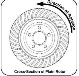
The rotors shown are all DRIVER/LEFT SIDE rotors. As you can see the surface slots rotate forward. Always be sure to install the rotors in this fashion. **NEVER INSTALL ROTORS IN THE OPPOSITE DIRECTION OF ROTATION**, heat related fatigue, and failure will result.
