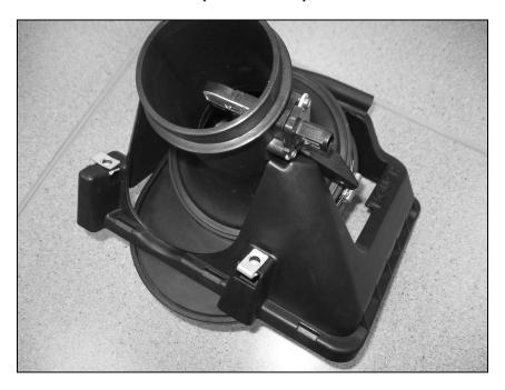
11. Install the EPDM close out seal (1111-9645) around the MAF Tube and clip into the edges of the upper air box tray.
