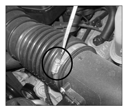
3. Loosen the hose clamp that connects the clean air tube to the intake.
