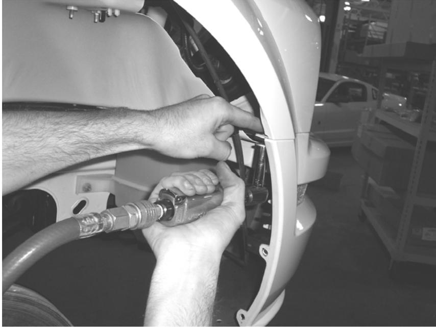
7. After all hardware has been removed, carefully remove front fascia from car by pulling the top corner down off of bolts. (Figure F)
