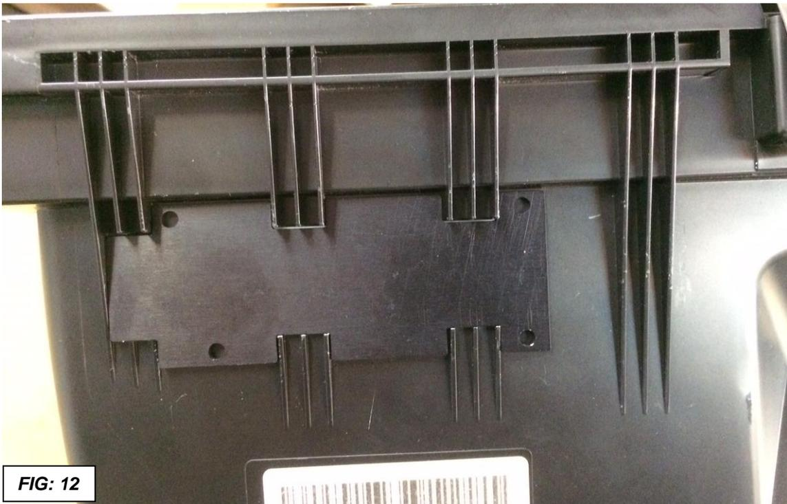
13. Using the cover plate as a drill template, drill the four hole pattern into the airbox using a #30 size drill bit. Install the 4 blind rivets in the hardware kit from the outside of the airbox.
