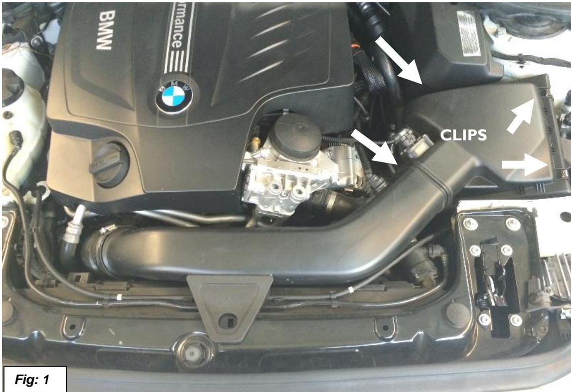
3. Gently unplug both the MAF sensor connection from the MAF sensor and the fuel tank breather valve. Some cars do not have this valve. See Figure 2.
