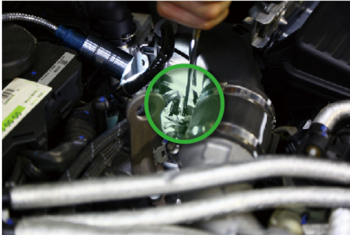
► 1. Remove the stock vacuum source
