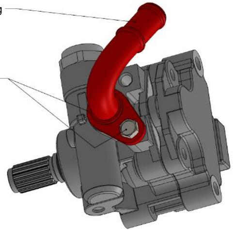
Sealing crush washers both sides
