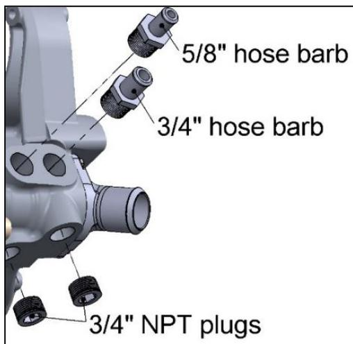
**Configurations:** On some swap applications there is not clearance for side heater hose outlets. There are optional bottom outlets for these applications.
