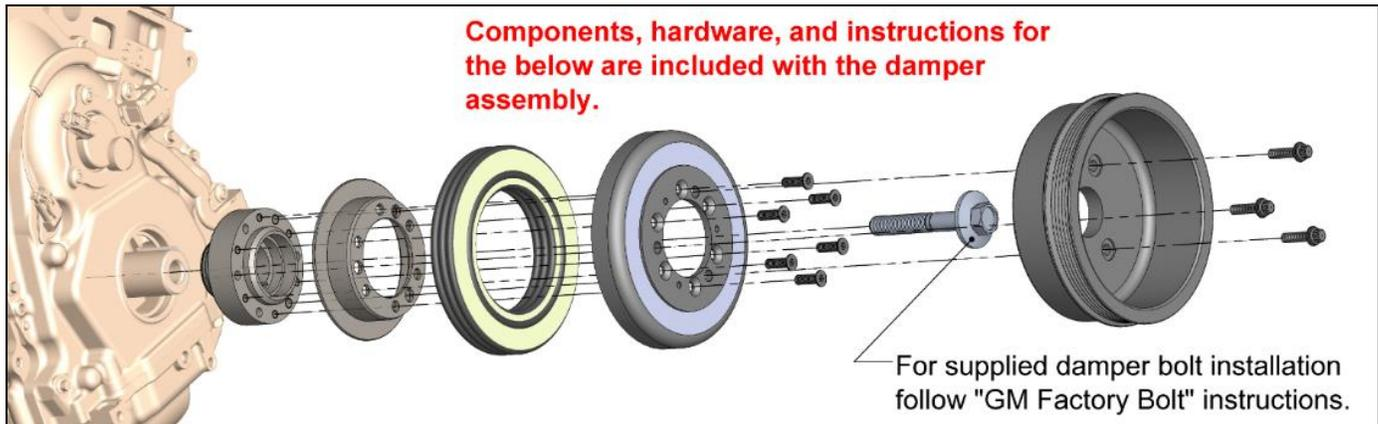
**HELPFUL HINT:** The above parts have a tight slip fit if aligned perfectly before assembly. If the aluminum pulley does not slip in the hub bore, the pulley can be placed in a freezer for 3 hours minimum. Remove and immediately install. Make certain the three pulley holes align to the hub while frozen because after the pulley warms you will likely not be able to rotate it in the hub.
