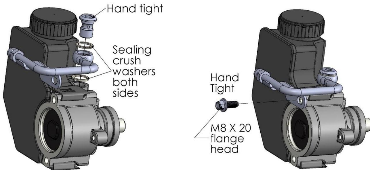
**NOTE:** After assembly torque M8 bolts to 18 ft./lbs. and banjo bolt to 25 ft./lbs.
