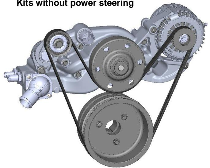
Holley's Mid-Mount complete accessory system has all accessories pulled in tighter than other accessory drives. Among the many swap friendly features is the bracket-less assembly that actually mounts all accessories to the water pump directly.
