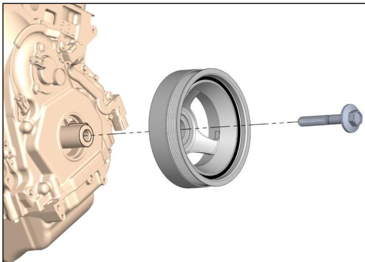
1. Remove original bolt (retain this bolt for later use)
