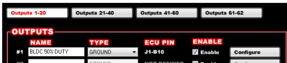
In this example configuration, the pump would run at 50% duty cycle when fuel flow is between 0 and 400 lb/hr. Above 400 lb/hr the ground output would be deactivated and the pump would run at 100%.
