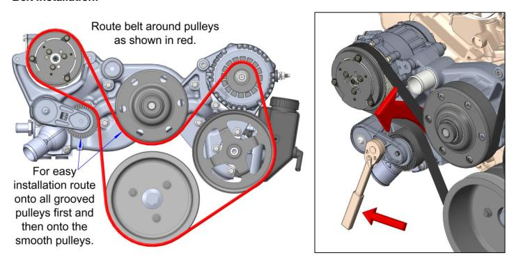
After routing the belt use a 1/2" square drive wrench to pull the tensioner all the way down and work the belt on from the rear.
