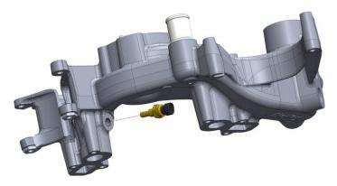
Install original temperature sensor removed from the LT water pump manifold. Torque to 15 ft./lb.
