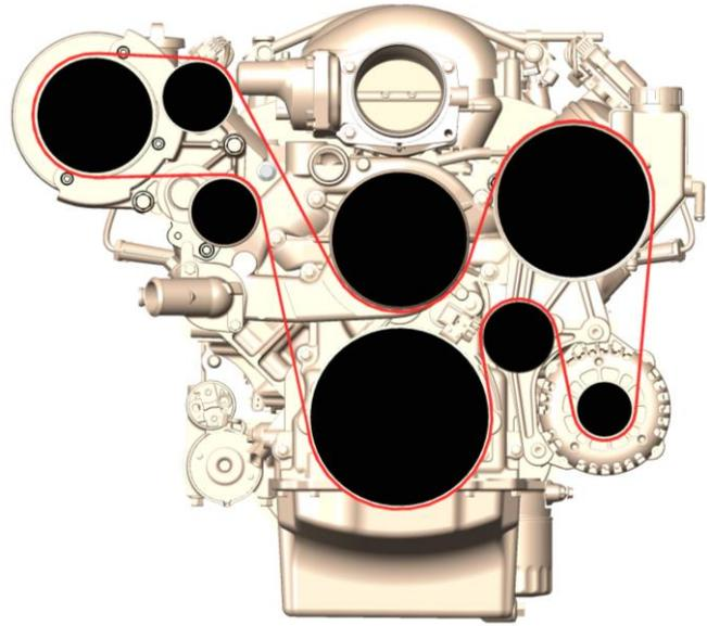
Alternate routing with AC bracket
