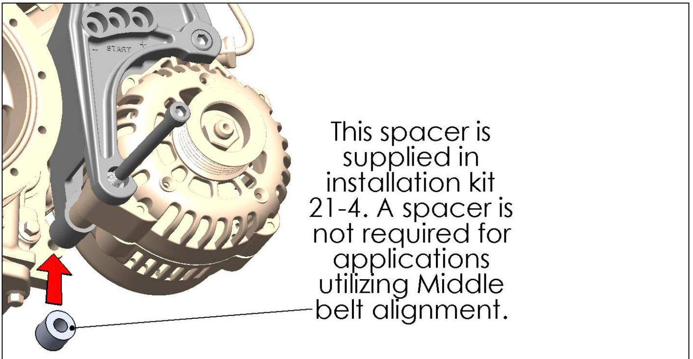
**NOTE:** Torque M8 bolts to 18 ft./lbs. and M10 bolts to 36 ft./lbs.
