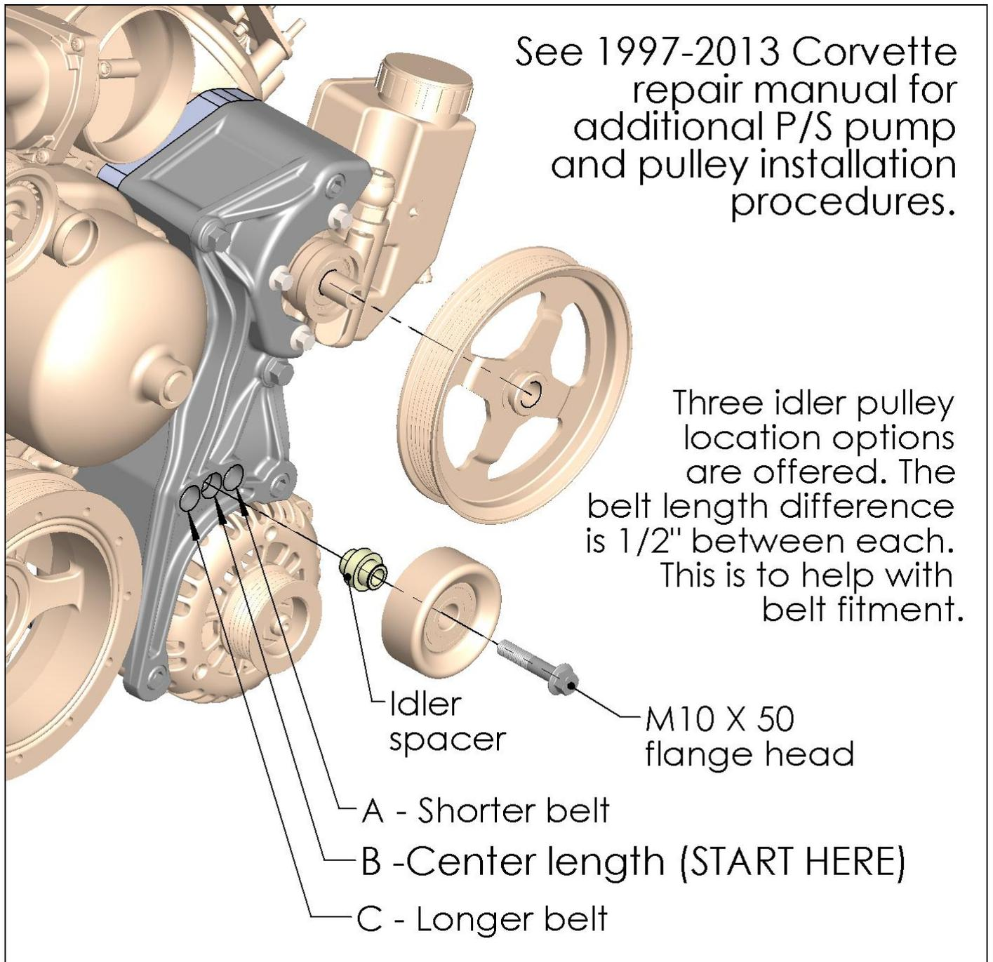
**NOTE:** Torque M8 bolts to 18 ft./lbs. and M10 bolts to 36 ft./lbs.
