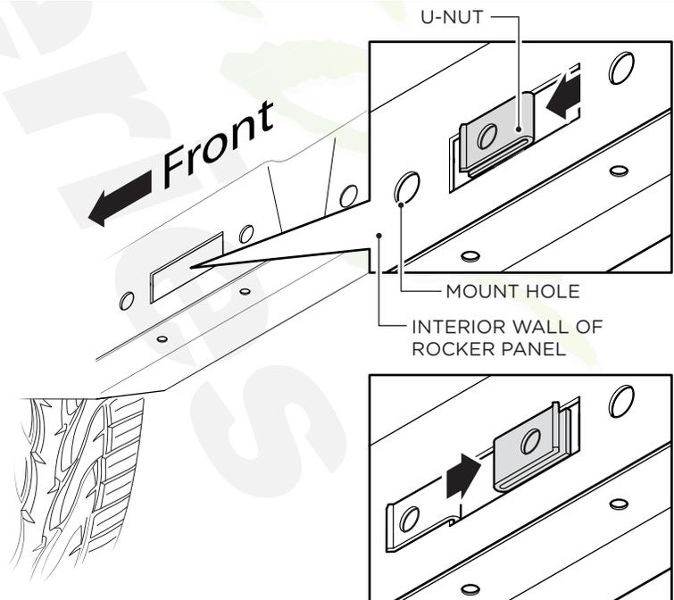
**3.** On the passenger side of the vehicle, align the Front and Rear Brackets as shown.
