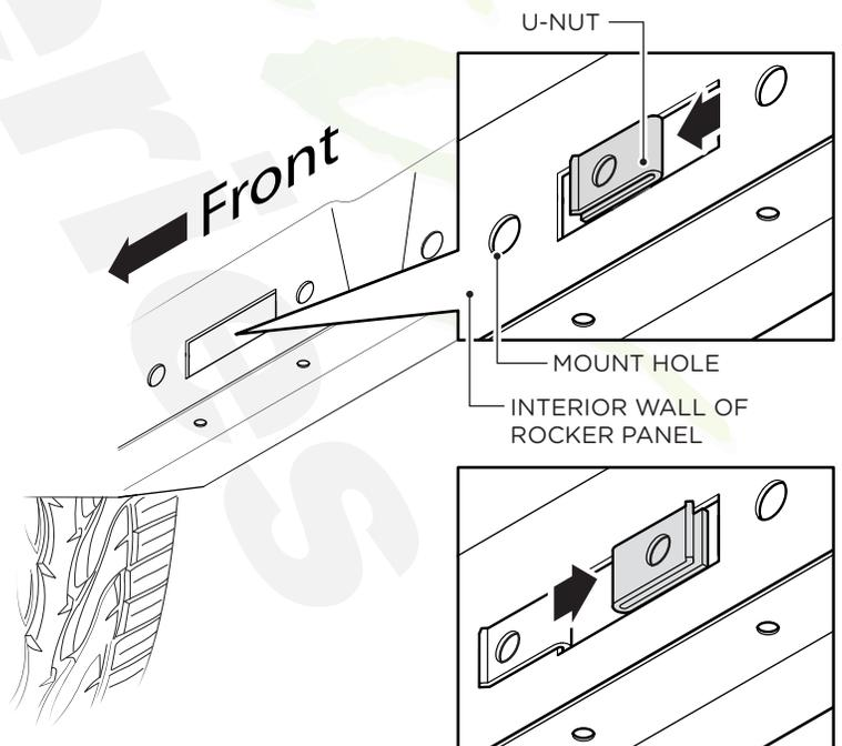
**4.** On the passenger side of the vehicle, align the Front and Rear brackets as shown.
