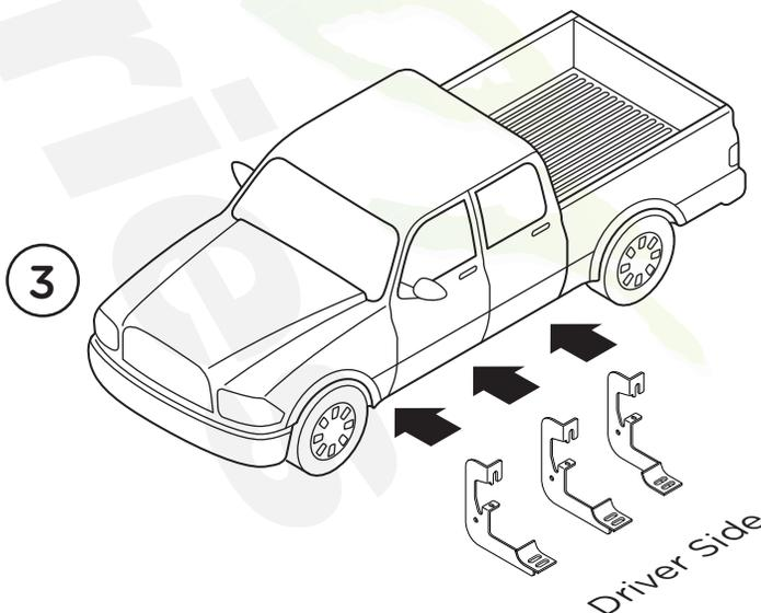
4. Existing mounting holes are located on the interior wall of the rocker panel. These mounting holes will be used per the following instruction.
