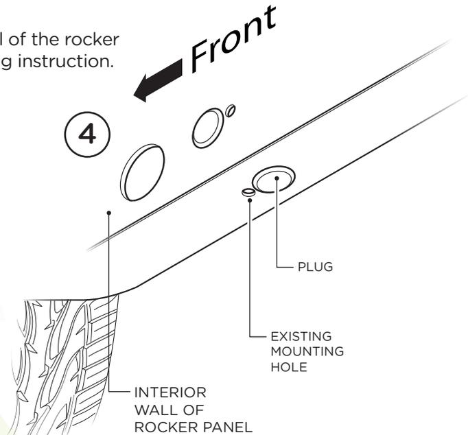
5. Remove the (2) plastic plugs from all (3) mounting locations in the rocker panel. Front Center and Rear. Insert M8 U Nut Clips so that the threads are on the inside of the rocker panel.
